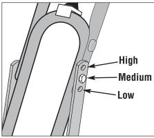
Figure 3-6: Handlebar height adjustment.
